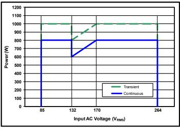
Figure 12: Rated output power vs Input AC Voltage.
