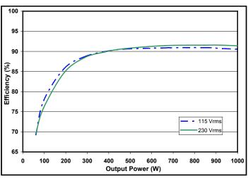
Figure 3: 15 VOUT efficiency curves.
