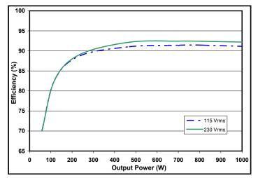
Figure 7: 28 VOUT efficiency curves.
