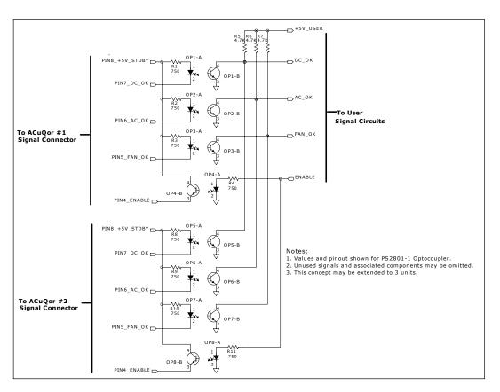
Figure P4: Isolated Signal Connections
