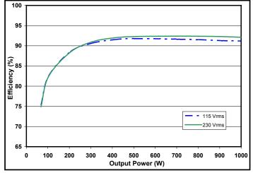
Figure 5: 24 VOUT efficiency curves.
