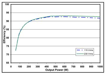
Figure 9: 48 VOUT efficiency curves.
