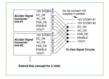
Figure P2: Simplest Signal Connections
