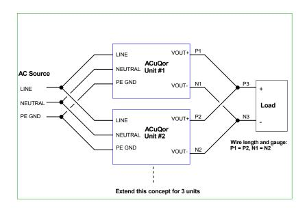
Figure P1: Parallel Power Connections
