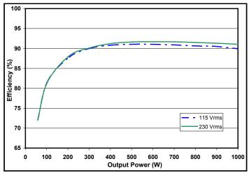
Figure 1: 12 VOUT efficiency curves.
