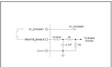
Figure B: Remote enable interface circuitry.
